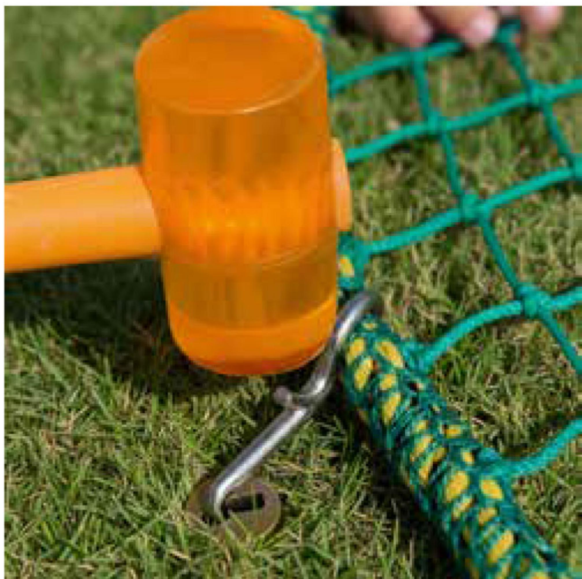
**C.** Tap lightly with a rubber mallet to ensure the anchor sits flush with the deck surface.
