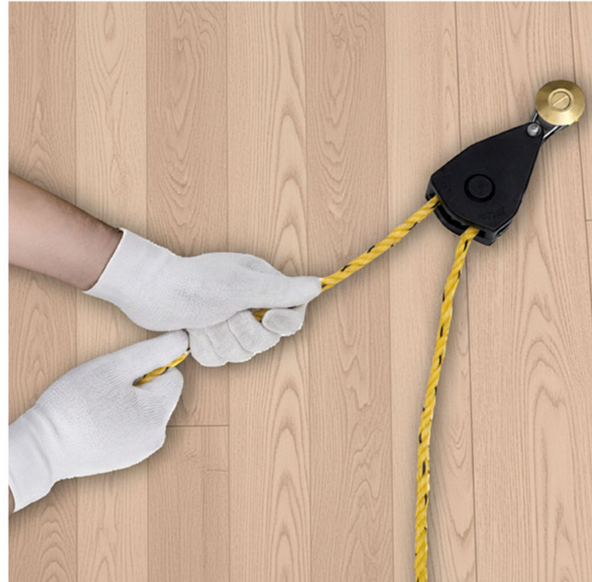
D. Secure the tensioner rope firmly by tightening the rope through the tensioner until the net is snug and even.
